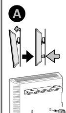
Place magnetic leveling feet 09 in the lower corners of the TV.
