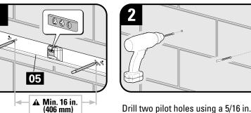
Drill two pilot holes using a 5/16 in. (8 mm) masonry drill bit.
