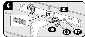
Install wall plate 05 with two washers 07 and screws 08, using bit 06. Securely tighten both screws 08
