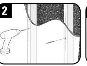
Drill two pilot holes using a 1/8 in. (3.2 mm) drill bit.
